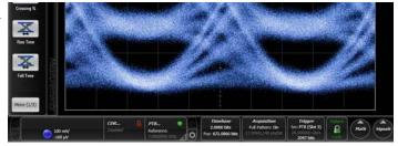
nominal amplitude resolution is 400  $\mu$ V and the amplitude accuracy is typically ±2.5% ±10 mV. The DC offset accuracy is typically ±20 mV.
